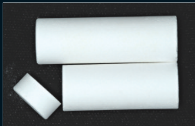
Fig. 4a and 4b. Sectioning disposable plunger from Microstar Corp to create Separating Buttons
