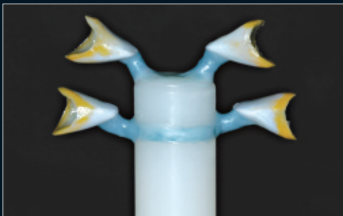
Fig. 1a and 1b. Spruing technique for two or three different shades
