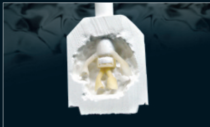
Fig. 8b. Cross section of two shades pressed prior to complete devesting
