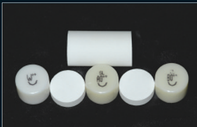
Fig. 6b. Larger plunger sectioned twice for pressing three different shades with 5-gram ingots
